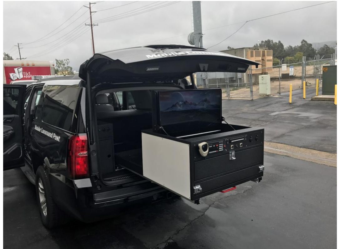
Command Slide Extended to access storage behind command desk and side dry erase boards
