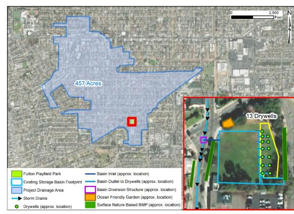
\* Nature-based BMPs may include bioretention, pervious pavement, and biofilters.
