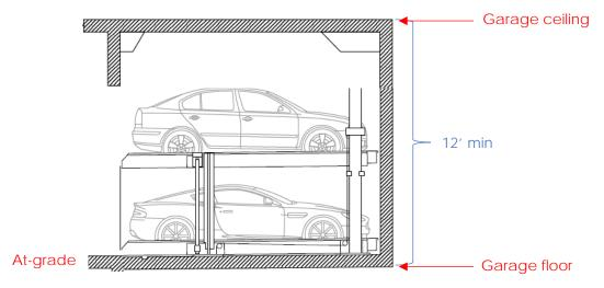
Example of vertical clearance from **below grade floor** to **the garage celling**:
