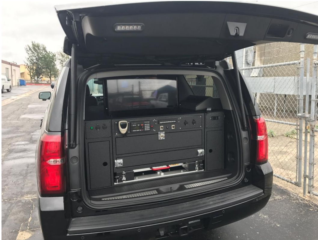
Rear Command Box with 32" HDTV Deployed inside vehicle
