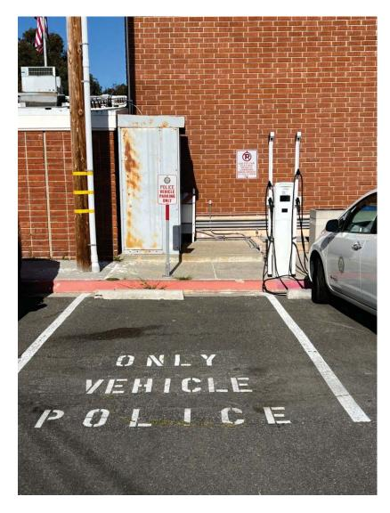
This project will explore the electrical power needs and installation of expanded electric vehicle charging infrastructure to serve the Police Department fleet on Bard Street, adjacent the Police Department and City Hall. The expanded charging would include up to 10 new chargers including both Level 2 and Level 3 chargers.
