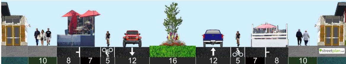
Figure 4. Hermosa Avenue - existing cross-section (looking north)
