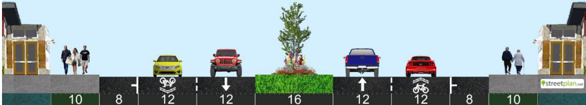
Figure 3. Hermosa Avenue - previous cross-section (looking north)
